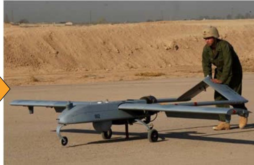
Assumed TUAS maximum payload with no degradation in ISTAR capability is 22kg
