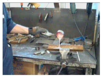
So we come to the possibility (our #4 above) of highly exothermic energy releasing reactions such as thermite (used here to include any aluminothermic reaction). Basic thermite is simply a mixture of aluminum powder and iron oxide. It's important to have it all in powder form so the iron oxide and aluminum particles will be in contact and react quickly. If you mix the powders thoroughly, and ignite them, the result is molten, white hot iron and a cloud of gray-white aluminum-oxide dust!
