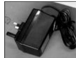
You should **never** use a so-called 'wall - wart' transformer like those used for phone chargers etc. They are unlikely to supply sufficient current and because they are unregulated they will cause a nasty buzz.
